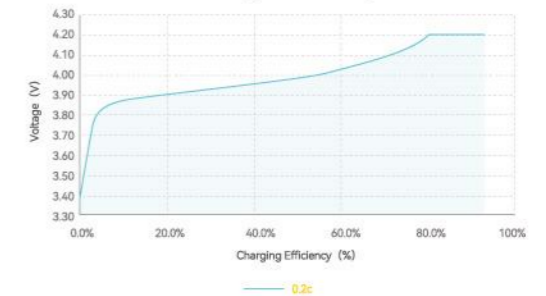
Low Temperature Battery Charging Curve 0.2C Charge To 4.2V @ -20^{\circ}\text{C}
