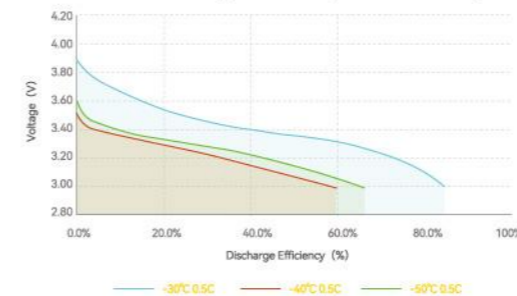
Discharge Curve At Different Temperature 0.5C Discharge To 3.0V ( -30^{\circ}\text{C} To -50^{\circ}\text{C} )
