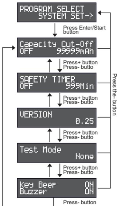
From the main charge menu press the "+/-" button to switch to "FUNCTION SELECT SYSTEM SET" position;
