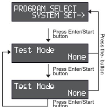
From the main charge menu press the +/- button to switch to the "PROGRAM SELECT SYSTEM SET" position
