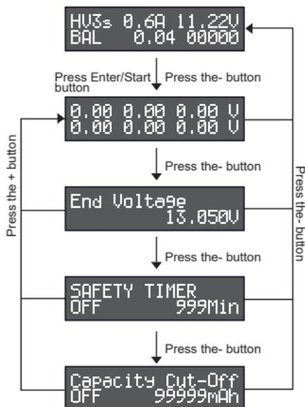
When working in the balance charge/cell balancing/storage/discharge mode, press the "+" button to check the voltage of each cell;
