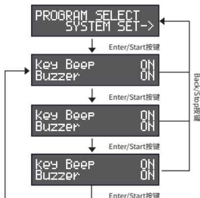
From the main charge menu press the +/- button to switch to the "PRPGRAM SELECT SYSTEM SET" menu
