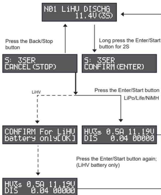
Select the battery chemistry, mode, cell count, amperage and other parameter settings (see details in 1.1 for parameter setting operation) to ensure that the parameters match the actual battery;
