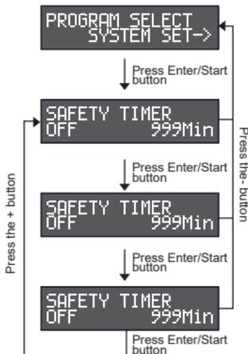
From the main charge menu press the "+/-" button to switch to the "PROGRAM SELECT SYSTEM SET" menu;
