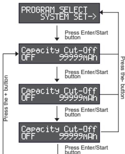
From the main charge menu press the "+/-" button to switch to the "PROGRAM SELECT SYSTEM SET" position.
