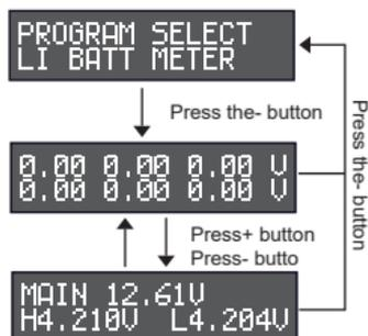
From the main charge menu press the "+/-" button to switch to the "PROGRAM SELECT BATT METER";
